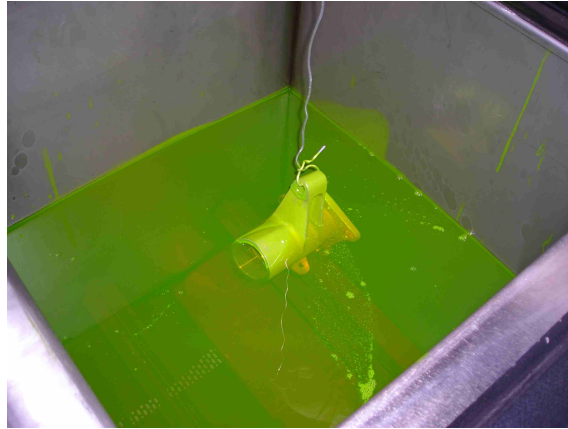
Fig. 5. Application of penetrant liquid.
