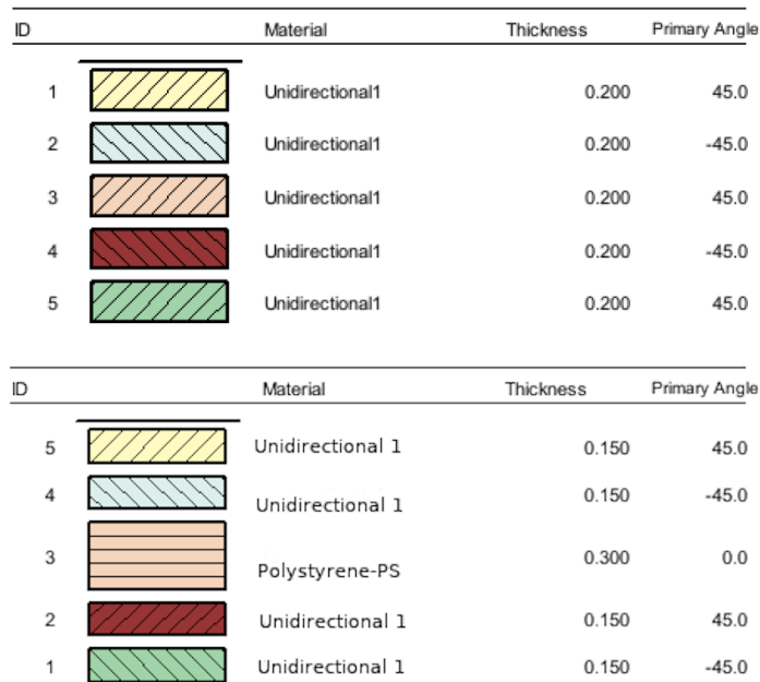
FIGURE 3. Structure of the laminate (top) and the sandwich (bottom).
