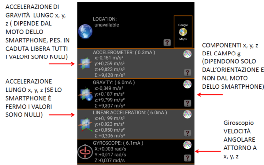
FIGURE 7. User interface of the “AndroSensor” APP. Note how the reading of the data collected in real time by the accelerometers is translated into the three quantities called respectively “ACCELEROMETER”, “GRAVITY” and “LINEAR ACCELERATION”.
