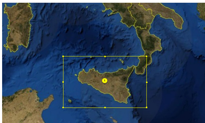
FIGURE 3. Map of the spatial domain used by the WRF model. The domain is centered on Sicily. The model is configured with horizontal grid spacing of 5km and a time interval resolution of 1h.
