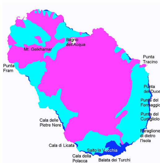
Figure 32. Schematic map of the eruptions pre and post green tuff, from Rapisarda (2007), based on the Pantelleria geological map of Orsi (2003). The flow of green tuff is shown in turquoise, while magenta indicates the surface affected by all successive lava flows. The areas in blue are the coastal zones where the layers prior to green tuff are accessible, because the sea erosion that created the cliffs tore the cover.
