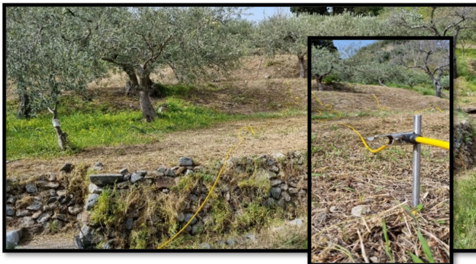
FIGURE 7. Photo of the survey line, with the magnification on an electrode planted in the ground.
