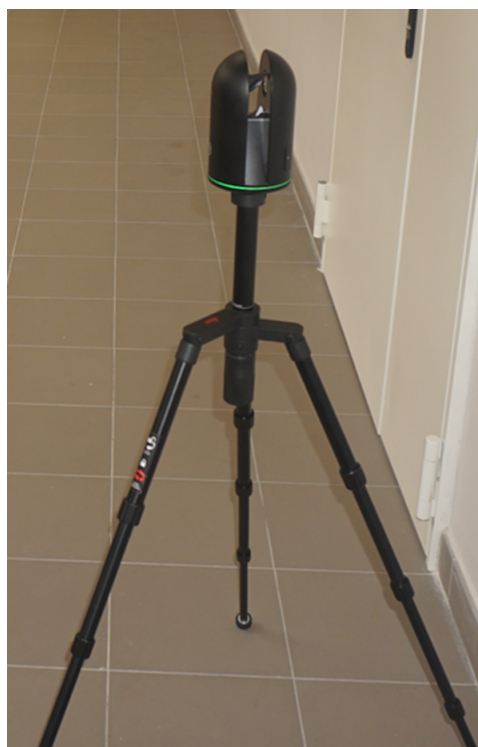
FIGURE 1. Leica BLK360 laser scanner of the Department of Engineering of the University of Messina.
