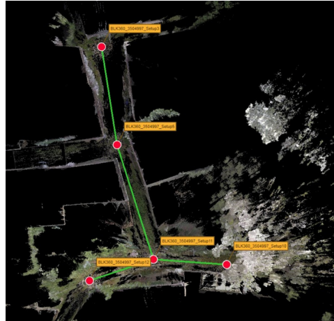
FIGURE 10. Case study No. 3: 2D map of the simulated crime scene with the position of the five scan stations and the station links (green line with error among 1 and 7 mm).
